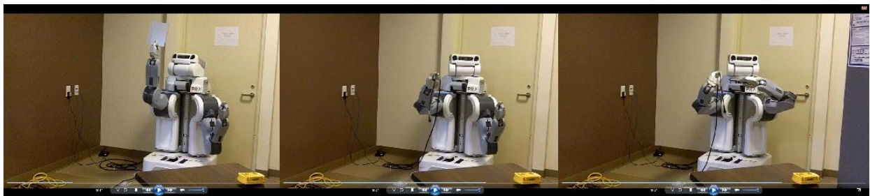
Figure 2: Robot Gesturing, (left) calibration imitation, (center) waving cord, (right) pointing at plug
